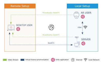
Fig. 9. System's architecture and implementation.<sup>3</sup>
