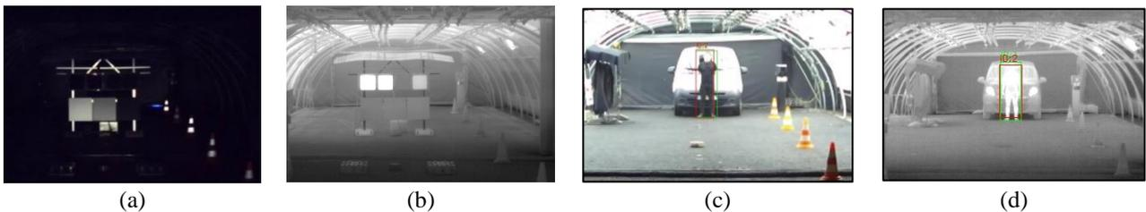
Fig. 3. Presentation of the different targets used during the test. From left to right : Scenario 1 with reference targets, for visible light (a) and thermal cameras (b), Scenario 2 with pedestrian and car, for visible light (c) and thermal cameras (d.)
