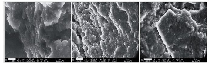
Figure 1. Scanning electron microscope images of  $Fe_3O_4$  (a), silica-coated nanoparticles (b), and MMIPs (c).
