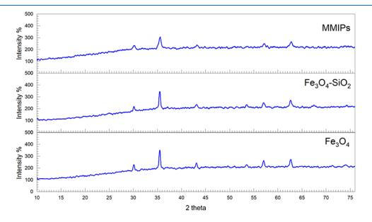
Figure 5. XRD graph of Fe<sub>3</sub>O<sub>4</sub>, silica-coated nanoparticles, and the magnetic molecularly imprinted polymer.
