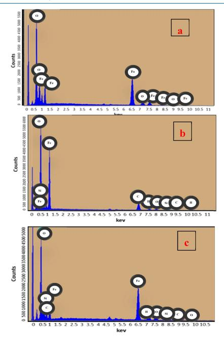
Figure 2. EDX diagrams of (a) Fe<sub>3</sub>O<sub>4</sub>, (b) silica-coated nanoparticles, and (c) the molecularly imprinted polymer.
