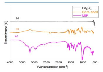
**Figure 4.** IR spectra of iron nanoparticles  $Fe_3O_4$  (a), core-shell (b), and the magnetic molecularly imprinted polymer (c).
