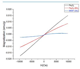
Figure 3. Vibrating sample magnetometer hysteresis loop of  $Fe_3O_4$ ,  $Fe_3O_4$ -SiO<sub>2</sub>, and MMIPs.
