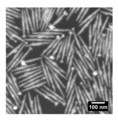
**Figure 1.** Structure of the functionalized azabodipy dye **1** and SEM images of the plasmonic nanostructures *AuBPs*@1730nm (the outline of one of the particles is enhanced with a dotted line to show the bipyramidal shape).
