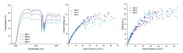
**Figure 8.** Transmission spectra, OPL and normalized OPL (respectively from left to right) of monoliths with concentrations of 56 mM in dye and 0.04, 0.08 and 0.16 nM in AuNPs (**Mlt-2** to **Mlt-4**) (Exc. 1550 nm).
