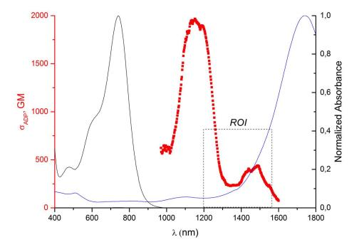
**Figure 2.** Overlay of normalized 1PA in dichloromethane (black) with 2PA (black squares) in carbon tetrachloride spectra of dye 1<sup>16</sup> and AuBP@1730 (blue) in water.
