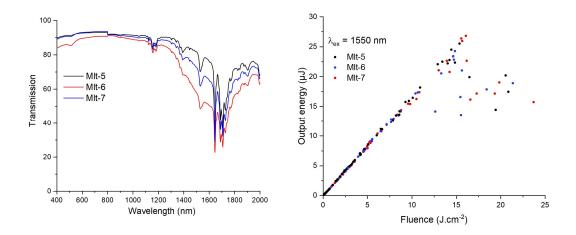
**Figure 6**. Left: Linear transmission of glass materials **Mlt-5** to **Mlt-7**. Right: Optical limiting of **Mlt-5** to **Mlt-7** doped solely with Au nanoparticles at concentrations of 0.04, 0.08 and 0.16 nM at 1500 nm.
