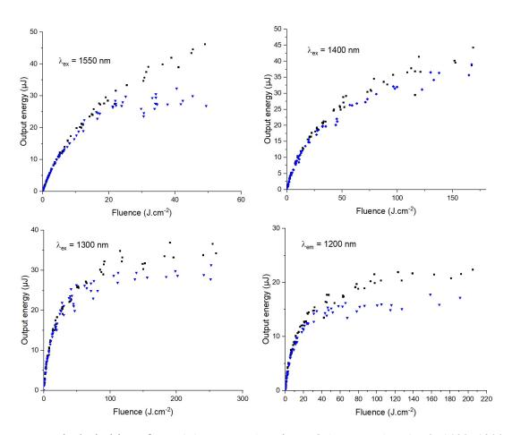
**Figure 7.** Optical Limiting of **Mlt-1 (black dots)** and **Mlt-3 (blue dots)** at 1550, 1400, 1300 and 1200 nm wavelength.
