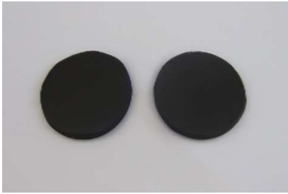
Figure 4. Different monoliths (from left to right, diameter 13 mm): Mlt-1 doped with dye 1 (5% wt) and Mlt-3 co-doped with dye 1 (5% wt) and AuBP@1730 (0.08 nM).
