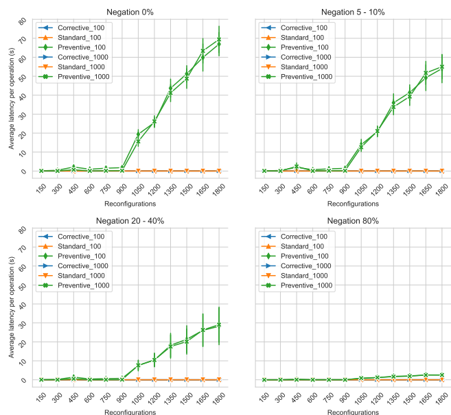
Fig. 9. Latency per reconfiguration operation, lower is better. Both the corrective and standard algorithms are instantaneous, while the preventive variant must wait. For 1800 concurrent reconfigurations the average latency per operation is 1 minute for preventive variant.
