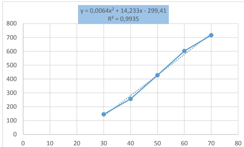
Diagram 7. The maximum amount of force per temperature for a muscle with a diameter of 0.8 mm
