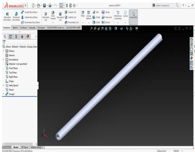
**Figure 6. Spring model of nylon muscle in SolidWorks**
