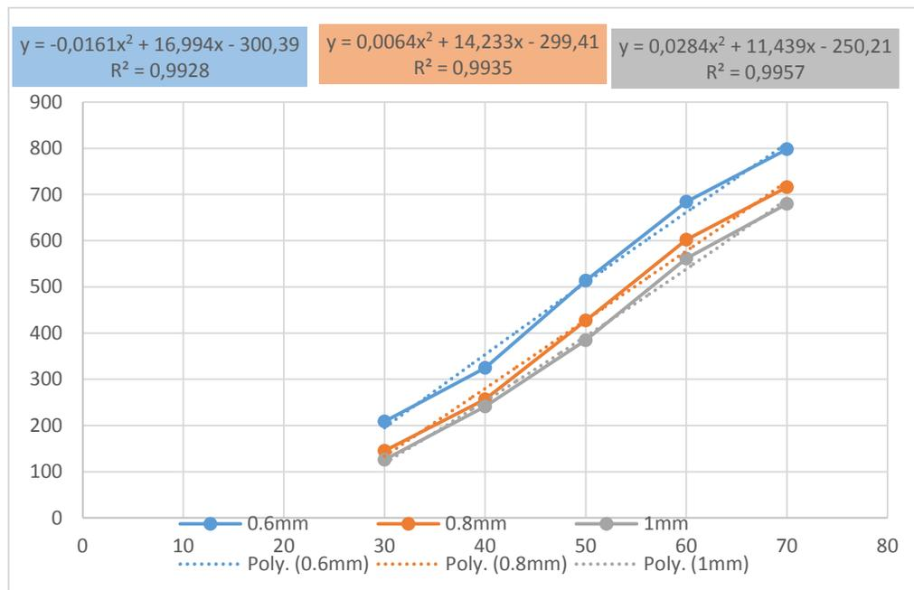
**Diagram 10. Comparison between the maximum amount of force in three diameters of 0.6, 0.8, and 1 mm**
