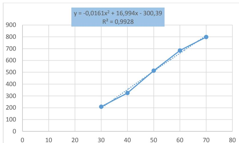
**Diagram 6. The maximum amount of force per temperature for a muscle with a diameter of 0.6 mm**
