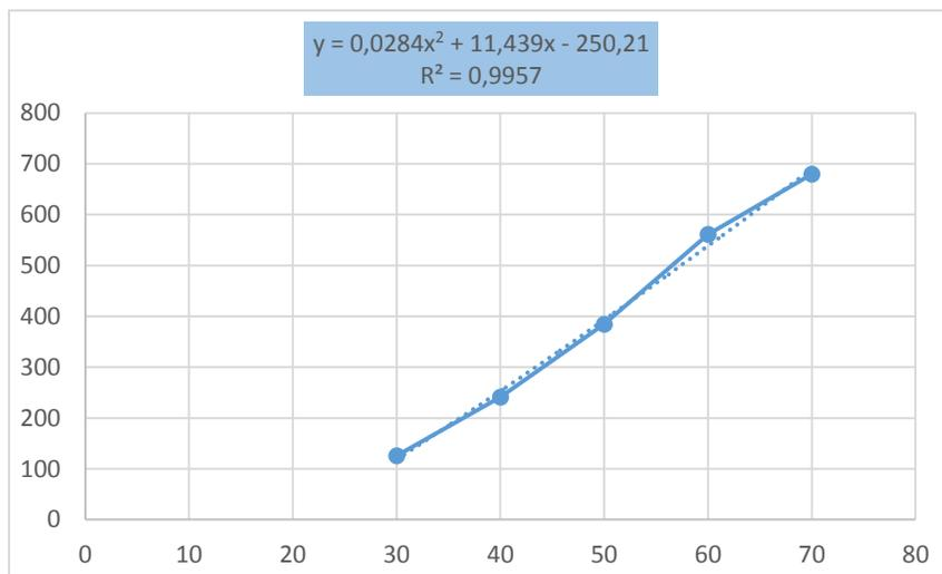
**Diagram 9.** The maximum amount of force at the temperatures for a muscle with a diameter of 1 mm
