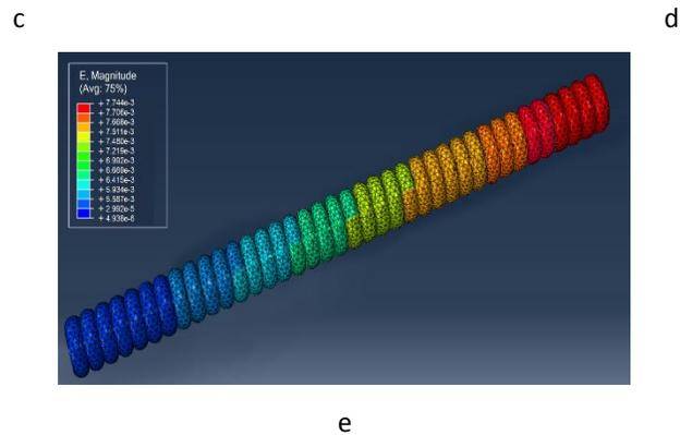
Figure 9. Muscle strain contour with a diameter of 0.8 mm; a) 30°C; b) 40°C; c) 50°C; d) 60°C and e) 70°C
