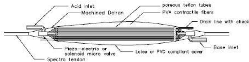
**Figure 4. Artificial muscle using a type of contractile gel [8]**
