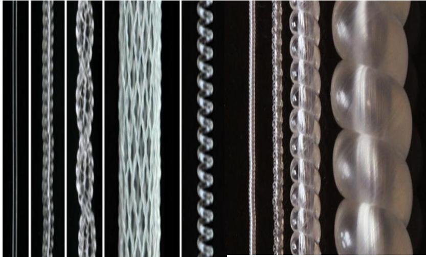
**Figure 1. Artificial muscles made of the nylon yarn**
