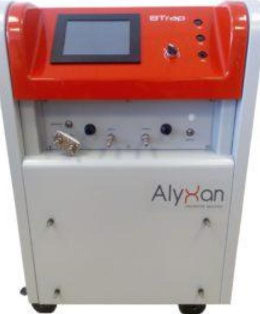
BTrap : The high mass resolution allows to separate quasi-isobaric compounds and to follow their evolution in the discharge. The chemical ionization can be done with two different precursors: either O<sub>2</sub><sup>+</sup> (to follow the n-hexane) or H<sub>3</sub>O<sup>+</sup> (to follow the by-products)
