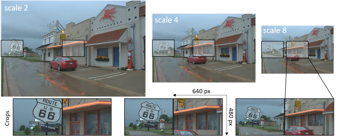
Fig. 1. Scale and Crop Strategy shows 66 Museum image taken from Fairchild’s HDR dataset [16]. The objective behind the strategy is natural augmentation of images for the dataset. The strategy creates three versions of each image, scaling the original size down by a factor of 2, 4 and 8 respectively. Consequently, for each version, a sliding-window crop of size 480 \times 640px is created with a horizontal and vertical stride of 100px .
