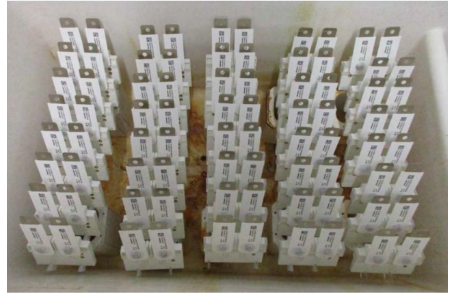
Fig. 4: A total of 40 samples are placed in a salt mist chamber for PD3 pre-conditioning. Half of the samples are protected while the other half are not.
