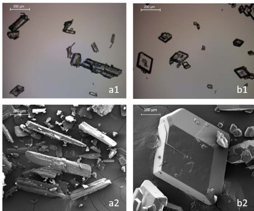
112 113 Fig. 1. OM (top) and SEM (bottom) micrographs of the stable \beta -form (a1, a2) and the 114 metastable \alpha -form (b1, b2) of L-Glutamic acid
