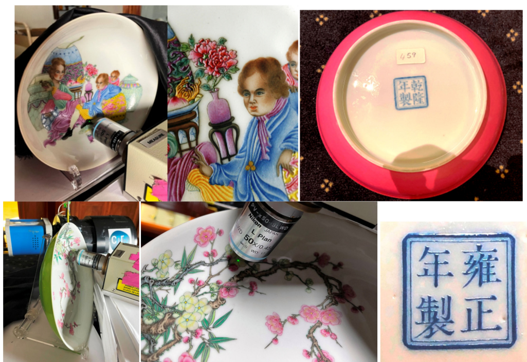
Figure 3. Views of the two dishes under Raman examination (top A608, bottom A596, see Table 1).
