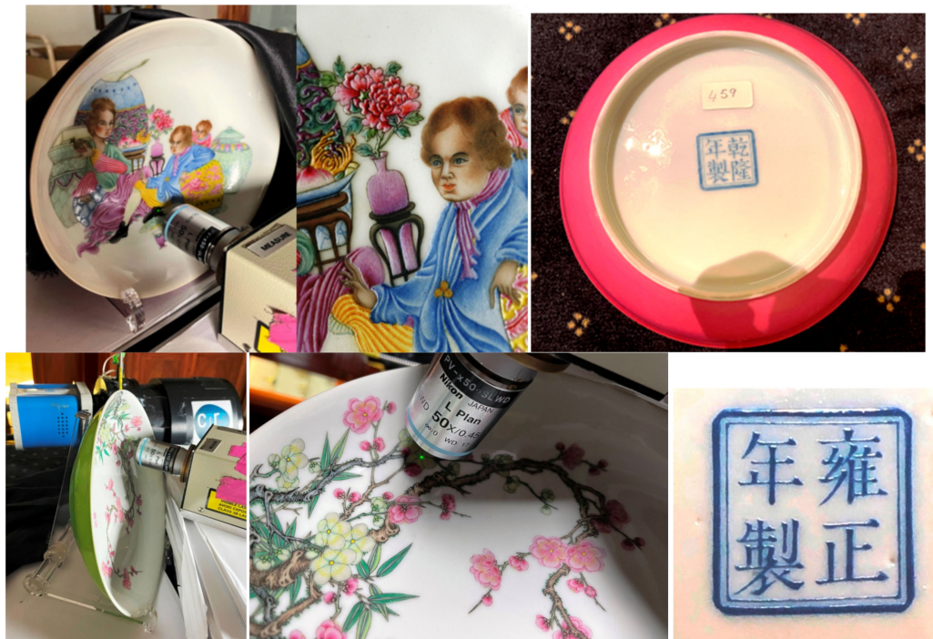
Figure 3. Views of the two dishes under Raman examination (top A608, bottom A596, see Table 1).
