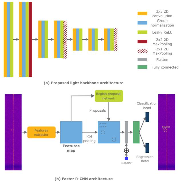
Fig. 2. Model architecture (lightweight Faster R-CNN architecture)
