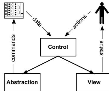
**Figure 2:** The three components of the Control-Abstraction-View software architecture model
