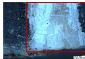
(b) Skin damages of 120% MC specimen
