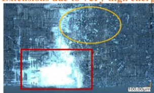
(a) Skin damages of dry specimen
