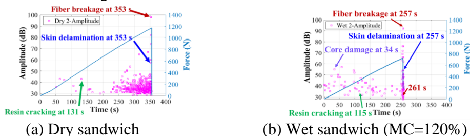
Fig. 4: Moisture effects on AE amplitude distributions of GFRP-balsa sandwich
