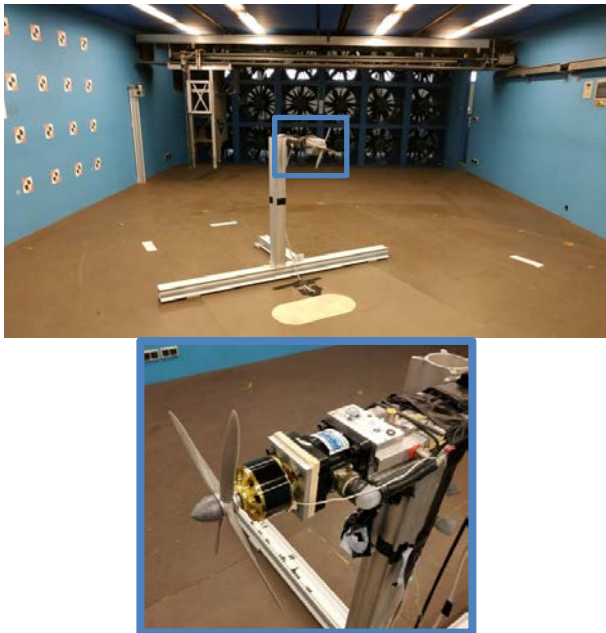
Figure 3 - Isolated small-scale propeller mounted in the L2 subsonic wind tunnel
