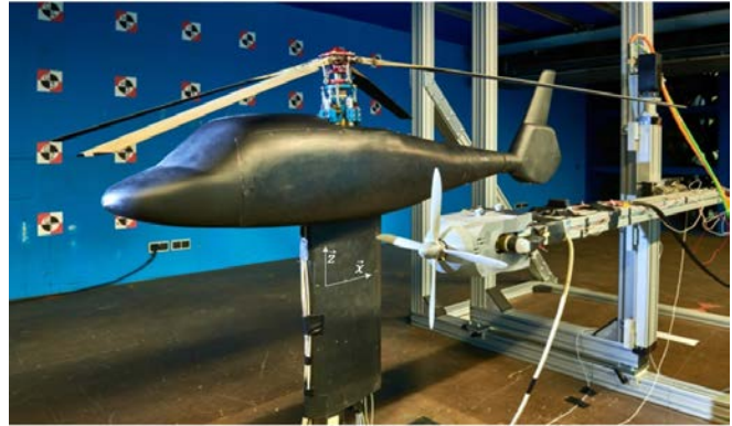
Figure 2 - Installation of the full assembly in the L2 wind tunnel
