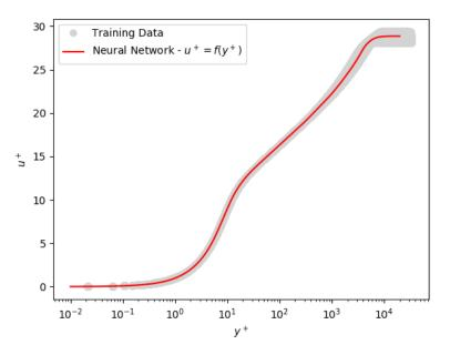
Figure 5: Network 1 (wall distance informed neural network): learned approximation of the dimensionless wall velocity  $\mathbf{u}^+ = \mathbf{f}(\mathbf{y}^+)$ .
