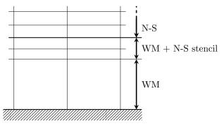
(b) Grid structure used for RANS simulations coupled with wall modeling and trimmed grid
