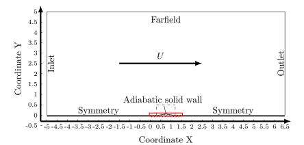
(a) Domain and boundary conditions for turbulent flow over the bump. The training dataset extraction is bounded by the dashed lines.
