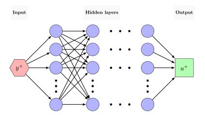
Figure 4: Network 1 (wall distance informed neural network): schematic diagram of the feedforward neural network with multiple hidden layers.
