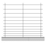
(a) Grid structure used for wall-resolved RANS simulations
