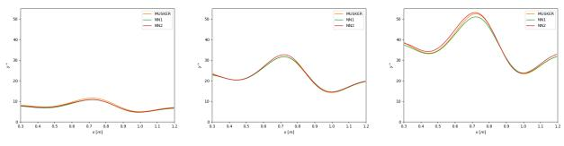
(a) Wall distance at first RANS computed cell (mesh labeled as  $\mathbf{y}^+ pprox \mathbf{10}$ ).
