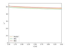
(a) Wall distance at first RANS computed cell (mesh labeled as  $y^+ \approx 10$ ).
