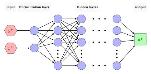
Figure 6: Network 2 (wall distance and pressure gradient informed neural network): schematic diagram of the feedforward neural network with multiple hidden layers.
