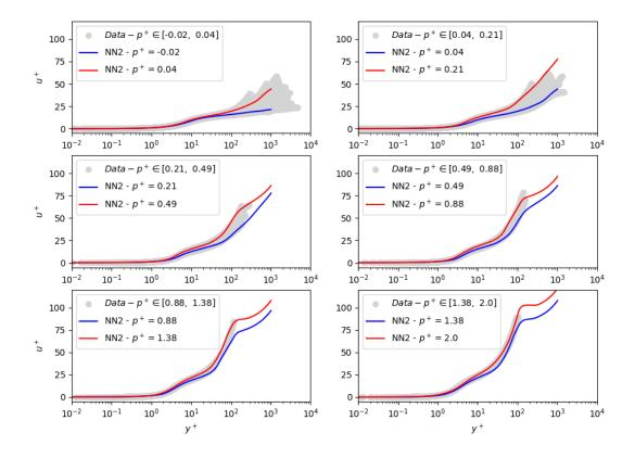
Figure 20: Learnt  $u^+ = f(y^+, p^+)$  relation by wall distance and pressure gradient informed neural network (Network 2).
