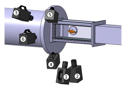
Figure 8: Sketch of the experimental configuration: camera positions and hydraulic tunnel. Cameras 3, 4, 5 and 6 were used for tomoPIV measurements.
