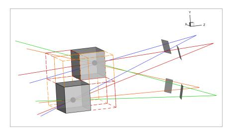
Figure 2: Illustration of the triangulation method used in this study. The volume is divided into boxes. For each box, and for each camera, the particles whose line of sight intersect the box are identified. If the box contains at least one line of sight for each camera, it is conserved, otherwise, it is eliminated from the list of boxes. When a conserved box contains more than one line of sight for at least one camera, it is divided into eight smaller boxes which are added to the list.
