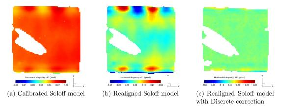
Figure 9: Maps of the horizontal component of the reprojection error for Camera 3, in the middle volume plane. The camera model is a polynomial (Soloff) model (degrees (3,3,2) in (X,Y,Z), with a discrete correction. (a) Model calibrated without correction (b) Model realigned without discrete correction (c) Model realigned with discrete correction
