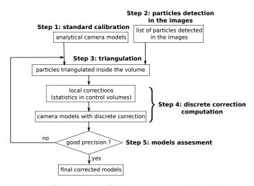
Figure 1: Algorithm of the camera model calibration
