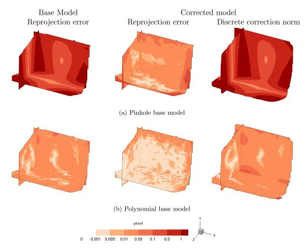
Figure 5: Maps of the reprojection error norm of the base model (left column), reprojection error norm of the corrected model (central column) and computed discrete correction norm (right column) for a pinhole base model (first row) and a polynomial base model (second row)
