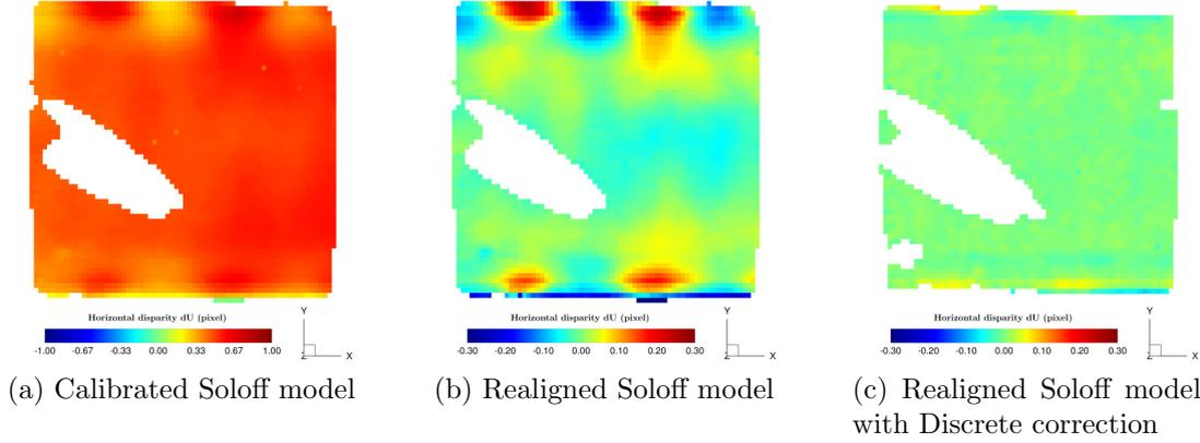
Figure 9: Maps of the horizontal component of the reprojection error for Camera 3, in the middle volume plane. The camera model is a polynomial (Soloff) model (degrees (3,3,2) in  $(X,Y,Z)$ , with a discrete correction. (a) Model calibrated without correction (b) Model realigned without discrete correction (c) Model realigned with discrete correction
