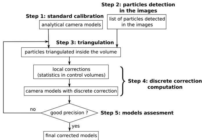
Figure 1: Algorithm of the camera model calibration
