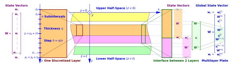
Figure 1: Geometry of the multilayer plate and state vectors. The discretization of each layer is described at the left-hand side, with the definition of the global state vector  $\mathbf{W}$  and local state vectors  $\mathbf{w}_0$  and  $\mathbf{w}_n$  at the bounds. The right-hand side summarizes how an inner interface is taken into account in the global state vector of the plate by introducing the additional interfacial state vector  $\mathbf{s}_I$ .
