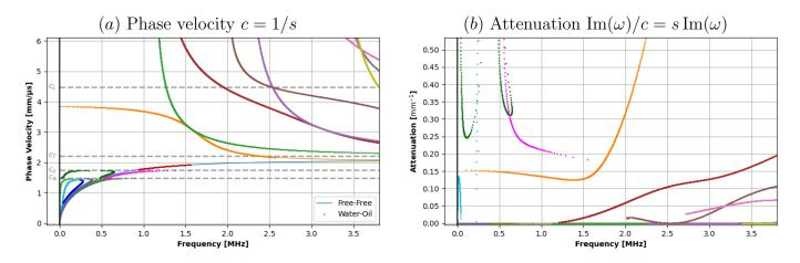
Figure 4: Fixed-slowness problem - water / 1 mm thick brass plate / motor oil: (a) phase velocities and (b) attenuations of modes versus frequency.
