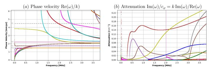
Figure 3: Fixed-wavenumber problem - water / 1 mm thick brass plate / motor oil: (a) phase velocities and (b) attenuations of modes versus frequency.
