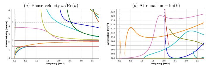
Figure 2: Fixed-frequency problem - 1 mm thick brass plate immersed in water: (a) phase velocities and (b) attenuations of modes versus frequency, to be compared with Fig. 7 of [18].
