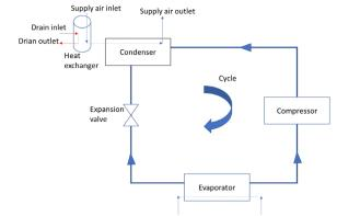
easily relying on an enhanced heat recovery ratio which is convenient for a better supply demand formula. Fig. 8 shows an example of a coupling between wastewater heat recovery system and w heat pump system. This drain system can be attached also to the evaporator.
