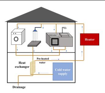
Fig. 2. Schematic of wastewater sources inside a house.
