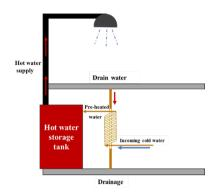
Fig. 5. Schematic of a vertical WWHR system assisted in a shower drain.
