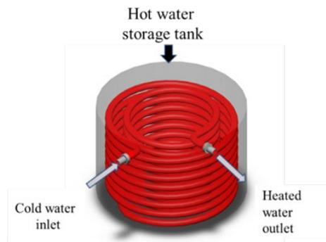
Fig. 6. Storage tank heat exchanger.
