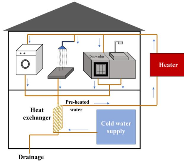
Fig. 2. Schematic of wastewater sources inside a house.
