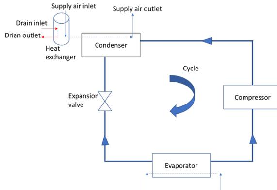
easily relying on an enhanced heat recovery ratio which is convenient for a better supply demand formula. Fig. 8 shows an example of a coupling between wastewater heat recovery system and w heat pump system. This drain system can be attached also to the evaporator.
