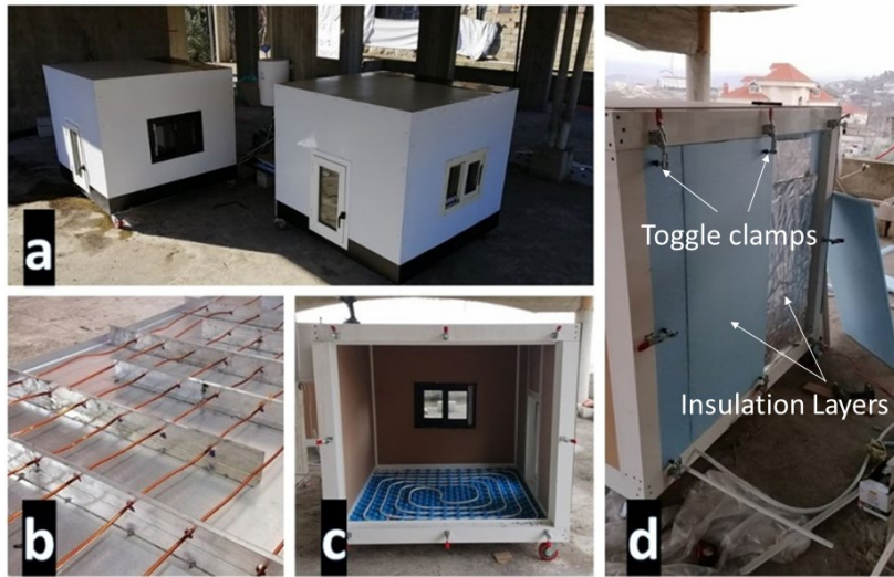
Fig. 2. (a) experimental setup of the two identical prototypes; (b) enhanced macro-container up on manufacturing; (c) underfloor heating system shown in the floor; (d) different layers being attached to the wall via hold-down toggle clamps.
