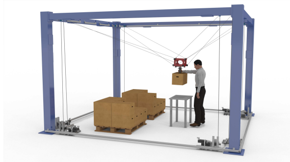
FIGURE 1 – A collaborative Cable-Driven Parallel Robot for manipulation task
