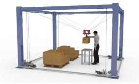
FIGURE 1 – A collaborative Cable-Driven Parallel Robot for manipulation task
