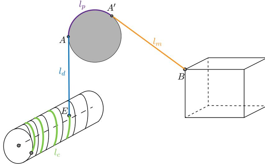
FIGURE 3 – Cable length in the actuation chain
