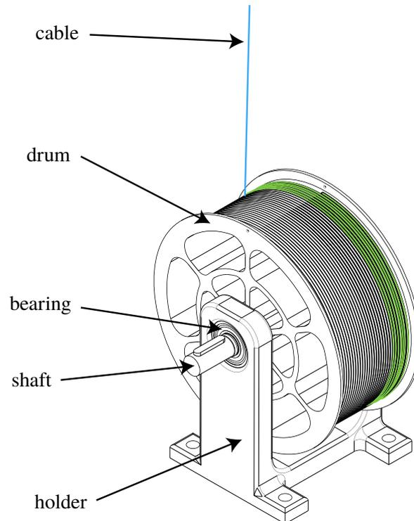
FIGURE 2 – Schematics of CRAFT reel and winch
