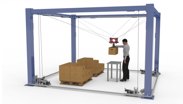
FIGURE 1 – A collaborative Cable-Driven Parallel Robot for manipulation task
