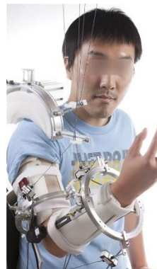
(a) CAREX rehabilitation robot [29, 30]
