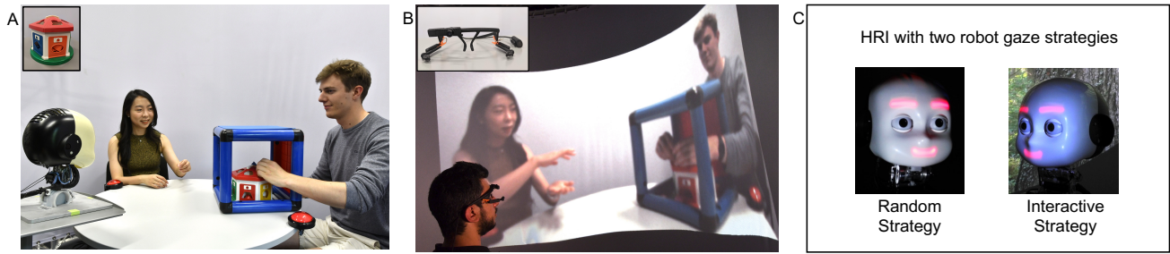
Fig. 1. Three tasks comprising our experimental setup starting with A) task 1 in which the robot remains static and records a pair of participants playing a cooperation game with a shape sorter (top left), followed by B) task 2 where the head and eyes of a participant watching the gameplay are recorded using an eye tracker (top left). In C) task 3 the robot performs movements based on either strategy while participants play the game described in task 1.
