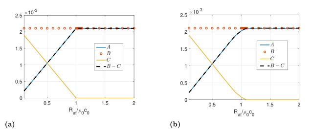
Figure 10. Plot of each term of the integral equation (8), with varying  $R_{at}$  from  $0.1\rho_0c_0$  to  $2\rho_0c_0$ , in case of no delay (a) and  $\tau = 2 \times 10^{-5}$  seconds (b). The other control parameters are set to  $\mu_M = \mu_K = 0.2$ .
