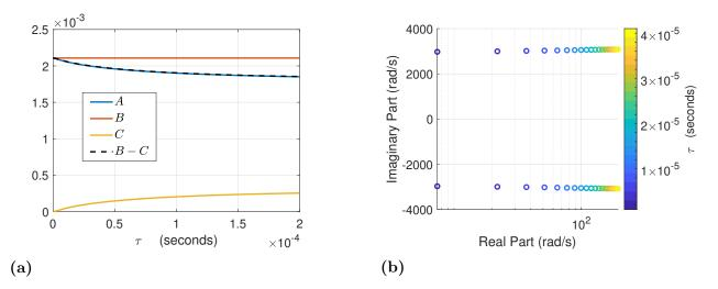
Figure 6. Plot of each term of the integral equation (8) (left) and of the unstable zeros of R(s) with positive real part, with varying time delay  $\tau$  from 0 to  $2 \times 10^{-4}$  seconds. The control parameters are set to  $\mu_M = \mu_K = 0.2$  and  $R_{at} = \rho_0 c_0$ .
