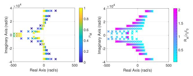
Figure 12. Closed loop poles migration with varying control parameters:  $\mu_M$  (left),  $R_{at}$  (right).
