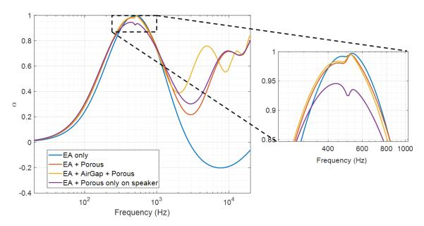
Figure 17. Simulated normal absorption of the EA only (in blue), of the EA plus a porous layer (in red), of the EA plus a porous layer with a 1 cm air-gap between them, and in case of porous layer applied just on the speaker (see Appendix C). The EA control parameters are:  $\mu_M = \mu_K = 0.2$ ,  $R_{at} = \rho_0 c_0$ ; the porous layer thickness considered is 12 mm with a flow resistivity  $\sigma = 1 \times 10^4$  rayl/m.
