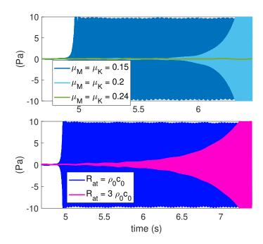
Figure 26. Time history of the pressure signal recorded at the upsurge of instability, for different values of  $\mu_M = \mu_K$  and of  $R_{at}$ , with the foam layer applied.
