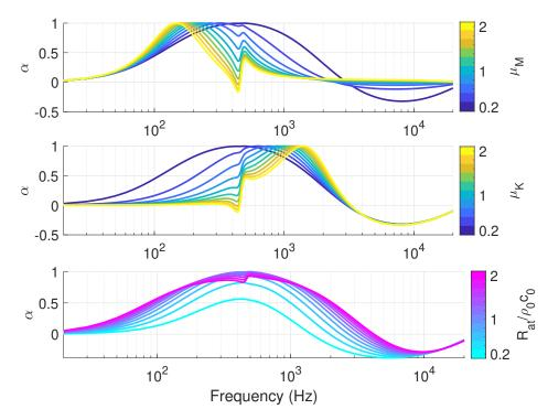
Figure 4. Variation of the absorption coefficient  $\alpha$  with respect to the control parameters, in case of a delay in the control loop equal to  $\tau = 2 \times 10^{-5}$  seconds. The default values chosen for the control parameters are  $\mu_M = 0.2$ ,  $\mu_K = 0.2$  and  $R_{at} = \rho_0 c_0$ .
