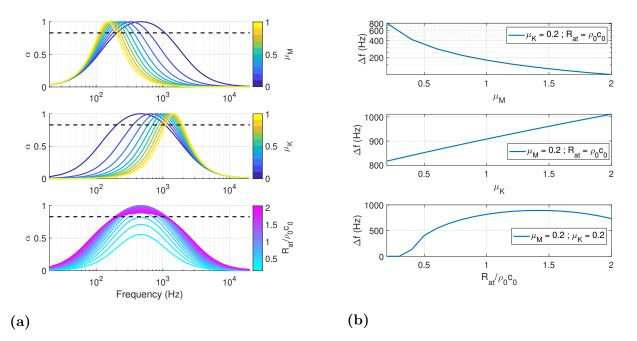
Figure 2. Variation of the normal absorption coefficient  $\alpha(\omega)$  (a) and absolute bandwidth  $\Delta f$  of efficient absorption (b) with respect to each of the target impedance parameters  $\mu_M$ ,  $\mu_K$  and  $R_{at}$ . The default values are  $\mu_M = 0.2$ ,  $\mu_K = 0.2$  and  $R_{at} = \rho_0 c_0$  respectively.
