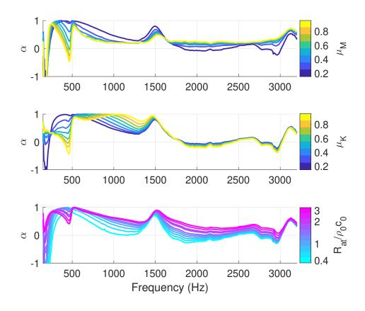
Figure 21. Variation of the measured normal absorption coefficient  $\alpha$  with respect to the control parameters, in case of a delay in the control loop equal to  $\tau = 2 \times 10^{-5}$  seconds. The default values chosen for the control parameters are  $\mu_M = 0.2$ ,  $\mu_K = 0.2$  and  $R_{at} = \rho_0 c_0$ .
