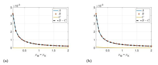
Figure 9. Plot of each term of the integral equation (8), with varying  $\mu_M = \mu_K$  from 0.1 to 2, in case of no delay (a) and  $\tau = 2 \times 10^{-5}$  seconds (b).  $R_{at}$  is set to  $\rho_0 c_0$ .
