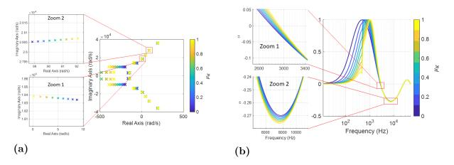
Figure 13. Effect of  $\mu_K$  on passivity (a) and stability (b).
