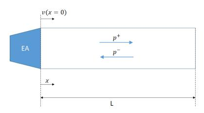
Figure 27. 1D hard-walled acoustic cavity with an EA on the left end and a rigid termination on the right end.
