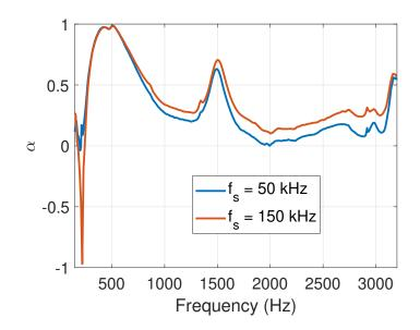
Figure 22. Measured normal absorption coefficient  $\alpha$  for two different sampling frequencies  $f_s$  and consequent time delays. The control parameters are  $\mu_M = 0.3$ ,  $\mu_K = 0.3$  and  $R_{at} = \rho_0 c_0$ .
