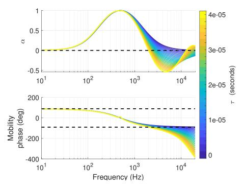
Figure 3. Absorption coefficient  $\alpha$  and mobility phase with varying time delay. The target impedance parameters are set to  $\mu_M = 0.2$ ,  $\mu_K = 0.2$  and  $R_{at} = \rho_0 c_0$ .
