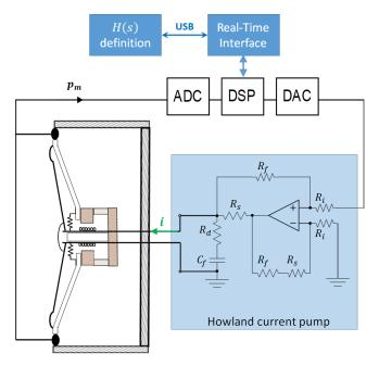
Figure 19. Scheme of the electronic components of the EA control.
