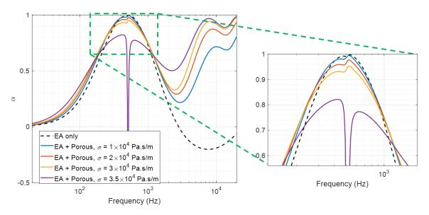
Figure 30. Effect of flow resistivity  $\sigma$  of a porous layer of thickness 12 mm, applied on the entire EA, on the absorption coefficient, with focus around resonance.
