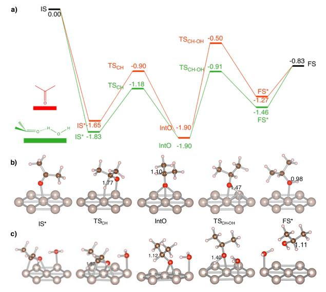
Figure 2: Acetone hydrogenation on Ru(0001) and H<sub>2</sub>O-Ru(0001) studied using the PW91 functional.<sup>56</sup> (a) Energy profiles in eV (b) Optimized structures on Ru(0001) (c) Optimized structures on H<sub>2</sub>O-Ru(0001). Main distances are indicated in Å.
