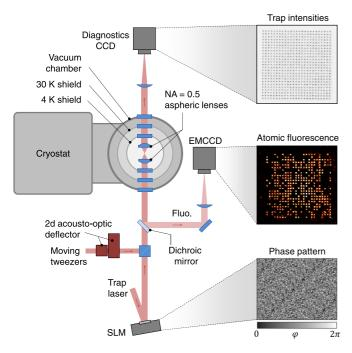
FIG. 2. Sketch of the experimental setup. The insets show, from bottom to top, the phase pattern used to produce a  $23 \times 23$  square array with a spacing of 5  $\mu$ m, an atomic fluorescence image of atoms loaded in the array, and an image of the trap intensities obtained on the diagnostics CCD camera.
