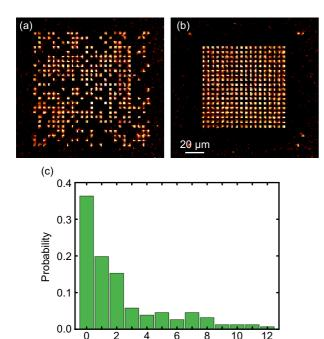
FIG. 5. Efficient assembly of a 324-atom array. (a) Fluorescence image of the 625-trap array before rearrangement. The lattice spacing is 5  $\mu$ m. (b) Fluorescence image of the array after two rearrangement cycles, showing a defect-free 324-atom array together with remaining reservoir atoms that have not been dumped yet. (c) Probability distribution of the number of missing atoms in the target array, showing a large ( $\simeq$  37%) probability of preparing *defect-free* arrays.
