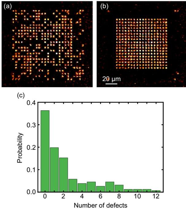
FIG. 5. Efficient assembly of a 324-atom array. (a) Fluorescence image of the 625-trap array before rearrangement. The lattice spacing is  $5 \mu\text{m}$ . (b) Fluorescence image of the array after two rearrangement cycles, showing a defect-free 324-atom array together with remaining reservoir atoms that have not been dumped yet. (c) Probability distribution of the number of missing atoms in the target array, showing a large ( $\simeq 37\%$ ) probability of preparing *defect-free* arrays.
