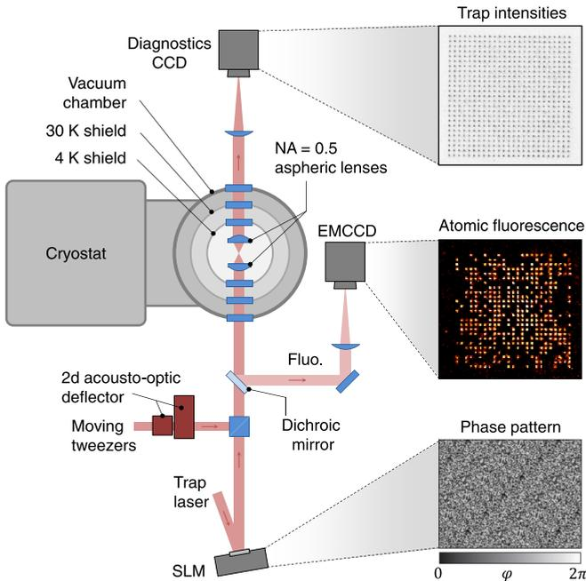
FIG. 2. Sketch of the experimental setup. The insets show, from bottom to top, the phase pattern used to produce a  $23 \times 23$  square array with a spacing of  $5 \mu\text{m}$ , an atomic fluorescence image of atoms loaded in the array, and an image of the trap intensities obtained on the diagnostics CCD camera.
