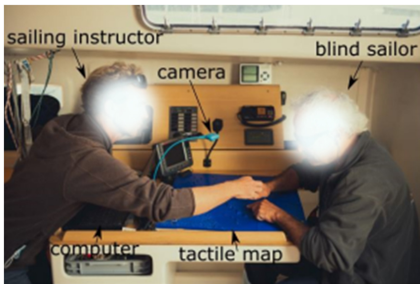
Figure 1. SMAug system at a chart table on a sailboat before navigation. The blind sailor consults the tactile map with a sticker on a finger to track it. Vocal announcements are triggered by the SMAug software. Thus, the sailing instructor and the blind sailor could prepare navigation together on the same map.
