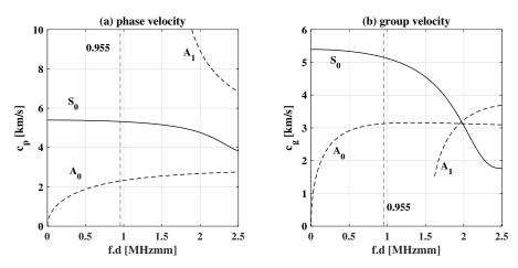
**Figure 5.** Dispersion curves of 2 mm thickness aluminium plate plotted using DC v2.0. The phase velocity curves are plotted to the left, whereas the group velocity curves are plotted on the right.
