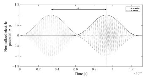
**Figure 15.** Time-of-flight  $\Delta t$  of  $S_0$  wave propagating, obtained from the electric potential ( $\Delta \Phi$ ) between sensor and actuator.
