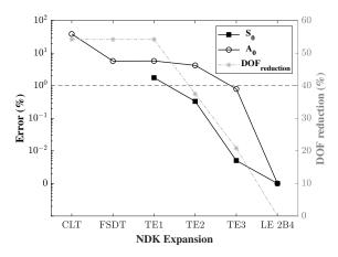
**Figure 22.** Assessment of the error in (%) in a node dependent kinematics model, with  $S_0$  and  $A_0$  wave propagation in an electro-mechanical plate model, compared to a refined full LE 2B4 model.
