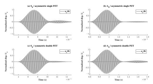
**Figure 19.** Showing the wave propagation in the electro-mechanical model at point B, for different wave natures and different sensor configurations.
