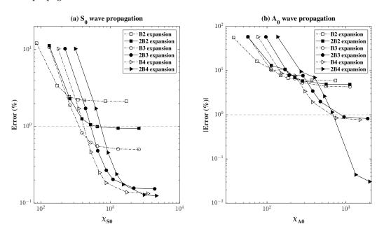
**Figure 16.** Error in (%) plotted in a log-log scale, for (**a**)  $S_0$  and (**b**)  $A_0$  wave propagation, using PZT actuators and sensor, as a function of  $\chi$ , for different model kinematics.
