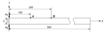
**Figure 4.** Boundary conditions and geometry of the mechanical plate model adopted for the propagation of Lamb waves, dimensions in mm.
