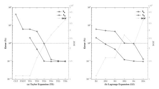
**Figure 11.** Assessment of the symmetric  $S_0$  and the antisymmetric  $A_0$  Lamb wave propagation under different through-the-thickness orders of expansion, in both (a) Taylor and (b) Lagrange models.
