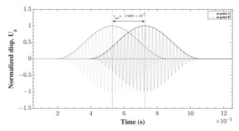
**Figure 7.** Analytical time-of-flight  $t_{ana}$  of  $S_0$  wave propagating between A and B.
