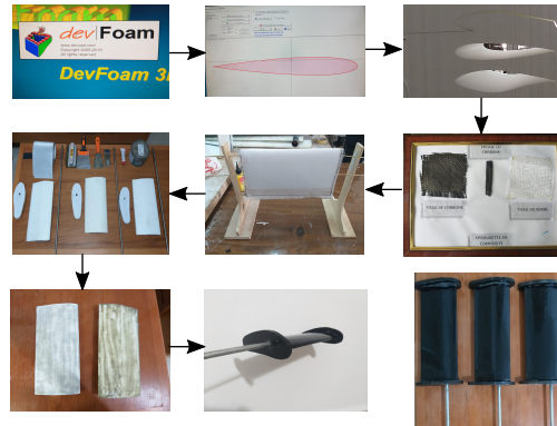
FIGURE 2 – Manufacturing process of the studied aerofoils.
