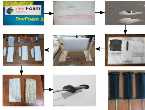
FIGURE 2 – Manufacturing process of the studied aerofoils.
