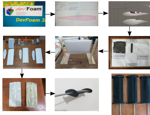
FIGURE 2 – Manufacturing process of the studied aerofoils.
