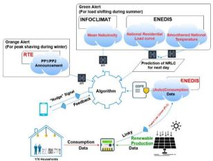
Figure 3: Schematic Diagram of project "EXPESIGNO"
