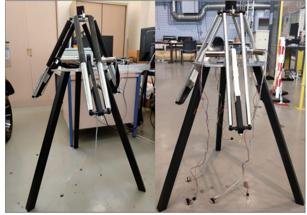
Figure 10: Real prototype in front view; left: Prototype Delta L for line-based visual servoing, right: Prototype Delta I for image moment visual servoing
