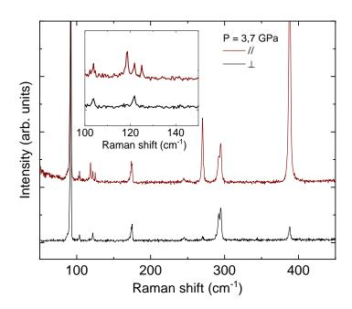
Figure S5. Linear-polarization resolved low temperature Raman scattering spectrum of bulk  $\text{FePS}_3$  at P = 3.7 GPa. The black (brown) line is the crossed- (co-) linear polarization configuration. Inset: Zoom on the magnon range of energy.
