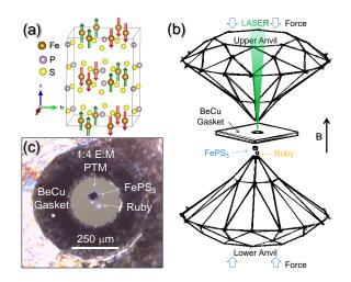
Figure 1. a) Crystal lattice of FePS<sub>3</sub> with the magnetic moments of the two zig-zag chains in green and red. b) Schematics of the experiment showing the diamonds of the diamond anvil cell, the FePS<sub>3</sub> sample and the ruby ball marker. c) Optical photograph of the pressure chamber showing the metallic gasket with a hole of diameter  $250\mu m$ .
