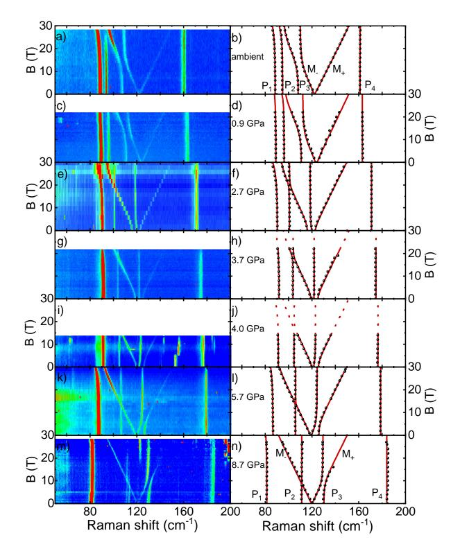
Figure 6. (left) False color maps of the magneto-Raman scattering response of bulk FePS<sub>3</sub> measured at T = 4.5 K and (right) evolution of the maxima of the peaks of the Raman scattering response (black dots) and of the calculated mode energies (red solid and dotted lines) as a function of the magnetic field for a,b) ambient pressure (from Ref. [16]), c,d) P = 0.89 GPa, e,f) P = 2.7 GPa, g,h) P = 3.7 GPa, i,j) P = 4.0 GPa, k,l) P = 5.7 GPa and m,n) P = 8.7 GPa.
