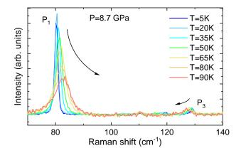
Figure 5. Evolution of the Raman scattering response as a function of the temperature at P = 8.7 GPa. The P<sub>1</sub> and P<sub>3</sub> phonons are indicated while the acquisition time does not allow for the observation of the weak P<sub>2</sub> and M features. The arrows are guides for the eyes.
