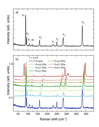
Figure 2. a) Low temperature (T = 4.5 K) Raman scattering spectrum of bulk FePS<sub>3</sub> measured at ambient pressure. The different phonon modes are labeled P<sub>i</sub> with i = 1 - 4 and F<sub>j</sub> with j = 1 - 4 and the doubly degenerated antiferromagnetic magnon excitation is labeled M. b) Low temperature Raman scattering spectra measured at different hydrostatic pressures up to P = 8.7 GPa with logarithmic scaling. Spectra are shifted for clarity.
