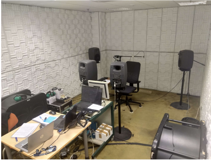
105 Figure 1: Photograph of the noise simulator in the sound restitution configuration for the acoustic experiment.
