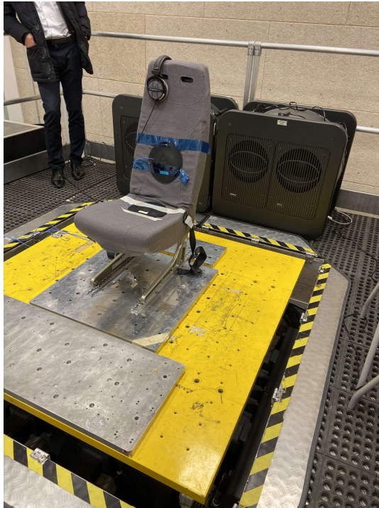
229 Figure 4: Experimental set-up for the experiment on the global sound and vibration discomfort.
