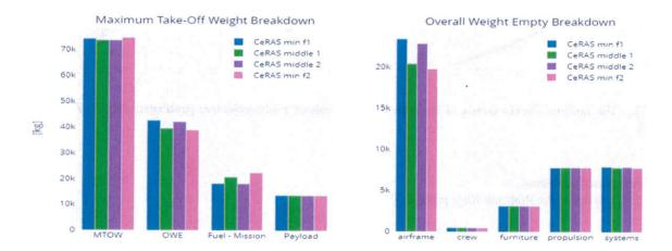
Fig. 11 Mass breakdown: Maximum TakeOff Weight and Overall Weight Empty for the four selected "CERAS" different configurations.
