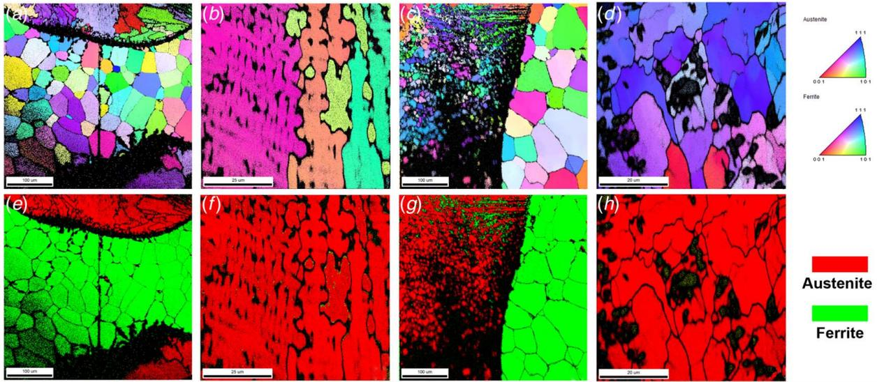
**Fig. 9** EBSD measurement of carburized zone section: (a) and (b) show IPF of sample at 75 W from both sides, (c) and (d) present IPF of sample at 100 W from both sides, (b) and (d) are magnified characterization in carburized zone of (a) and (c) respectively, and (e)–(h) show the phase distribution of (a)–(d)
