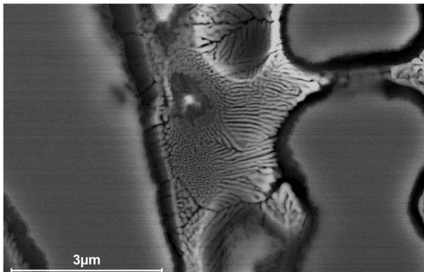
**Fig. 8 SEM image of an interdendritic region**
