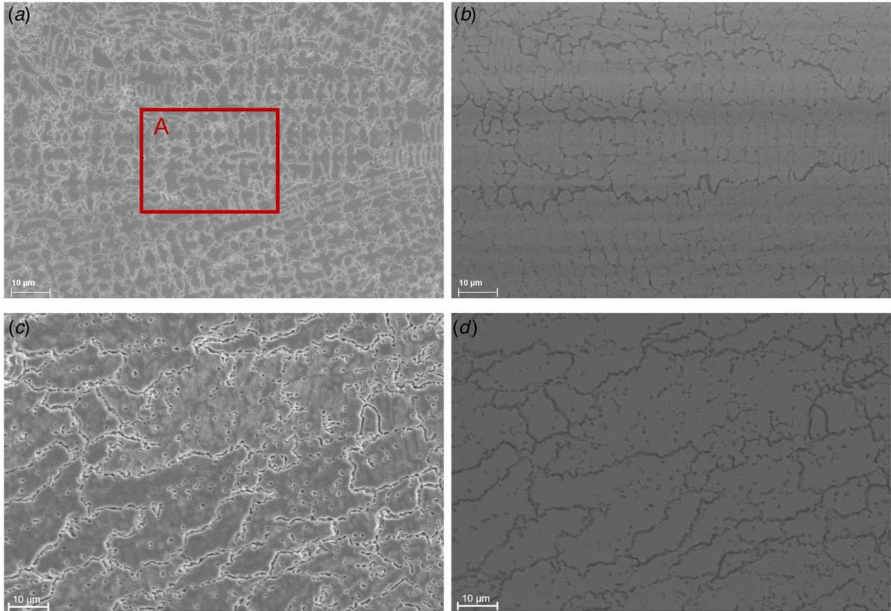
**Fig. 6** SEM images of LC samples at (a) and (b) 75 W on both sides, (c) and (d) 100 W on both sides, (a) and (c) SE signal, (b) and (d) BSE signal
