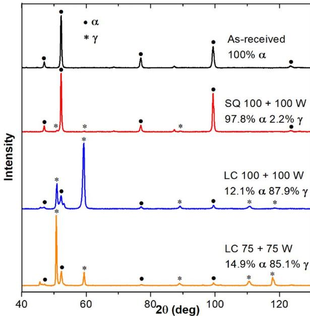
**Fig. 10** XRD patterns and phase composition of samples treated under different conditions
