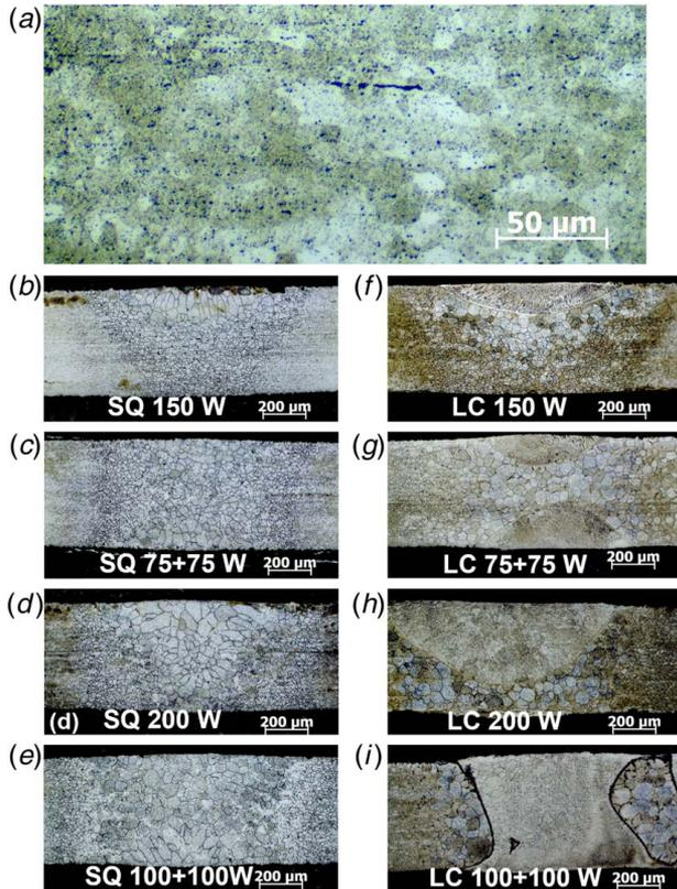
**Fig. 4** General section microstructure of (a) as-received material, (b)–(e) SQ samples, and (f)–(i) LC samples
