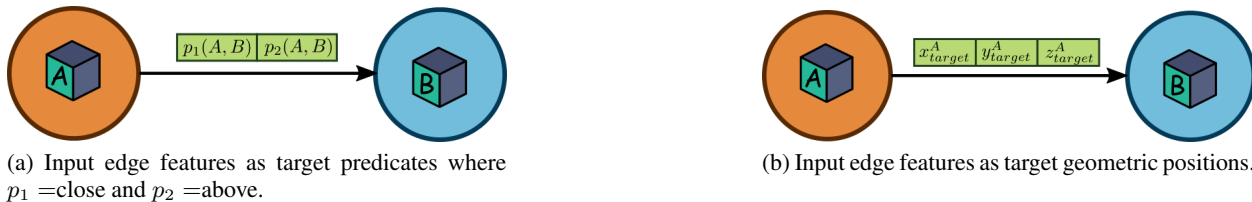
Figure 2: Illustration of a single directed edge for semantic goals (a) and continuous goals (b).
