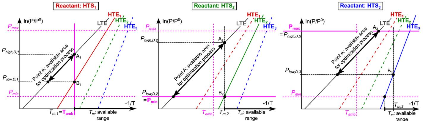
Fig. 6 – Process used to define the main temperature and pressure levels of the autothermal step, highlighted for three reactive salts (temperature pinches are neglected).
