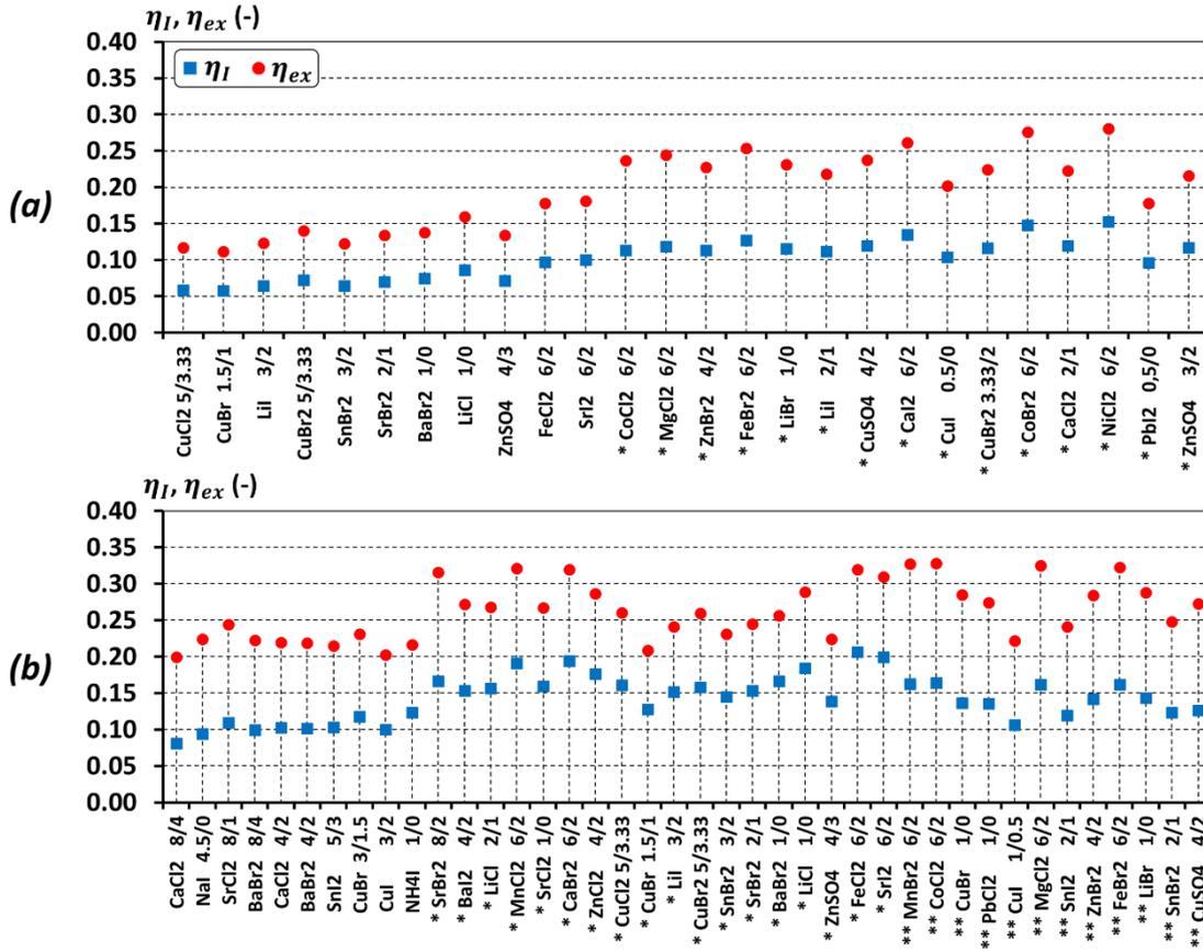
Fig. 10 – Discharge power generation mode: energy and exergy efficiencies of the cycle for selected salts.
