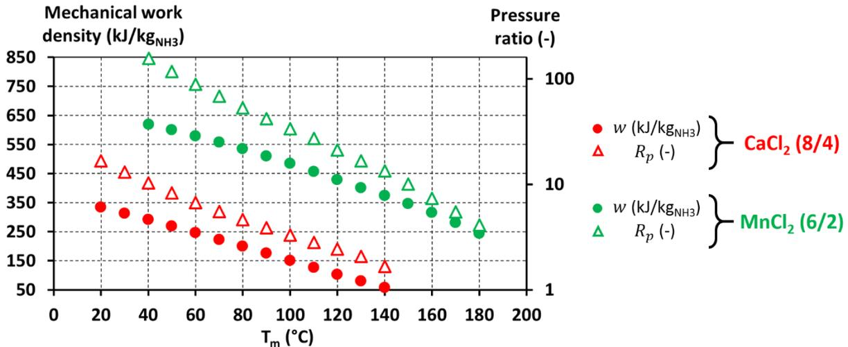
Fig. 7 – Influence of the temperature level  $T_m$  of the autothermal discharging step on power production: mechanical work density  $w$  (left scale, circles) and pressure ratio  $R_p$  (right scale, triangles).
