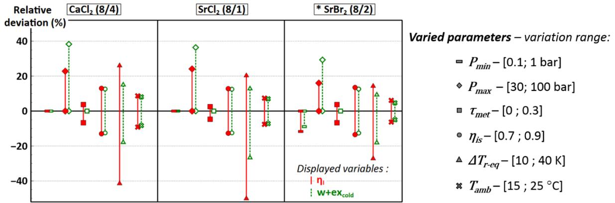
Fig. 16 – Sensitivity analysis for combined charge and discharge power generation mode (single sorption cycle). Symbols are the extremal relative deviations of  $\eta_I$  (red) and  $w+ex_{cold}$  (green) with respect to their nominal values: minimal and maximal values of  $\Delta(\eta_I)/\eta_{I,nom}$  (red symbols) and  $\Delta(w+ex_{cold})/(w+ex_{cold})_{nom}$  (green symbols)
