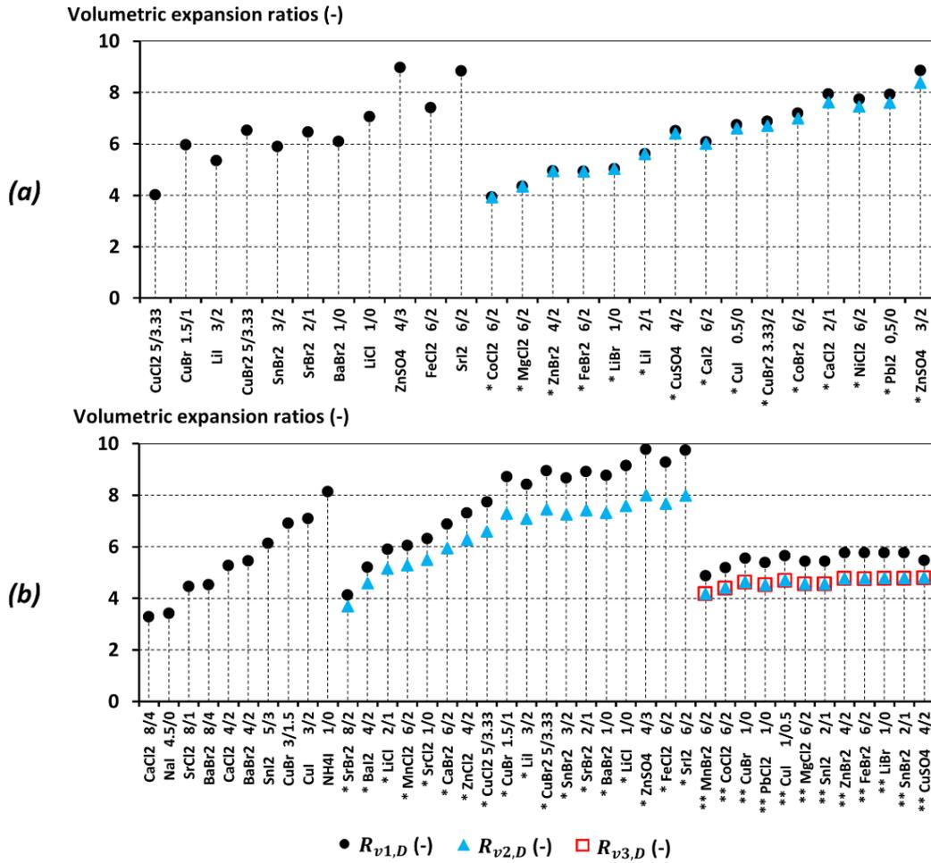
Fig. 9 – Discharge power generation mode: operating conditions of the hybrid cycle for selected salts (volumetric expansion ratios).
