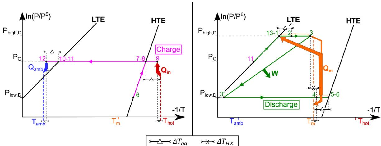
Fig. 2 – Discharge power generation mode of the hybrid thermochemical cycle: thermodynamic path in a Clausius-Clapeyron diagram (Left side: charging step. Right side: discharging step). For the sake of clarity, the switching step between charging and discharging steps is displayed in a simplified way (considering only points 6 and 11 on the equilibrium lines)
