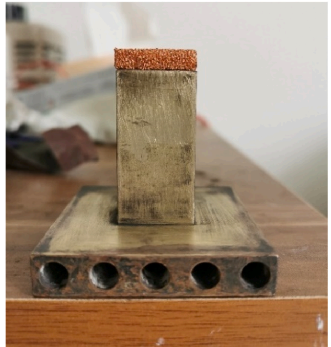
Fig. 4. Metal foam soldered to a heated copper block.
