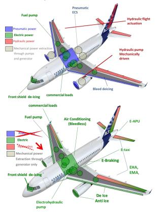
Figure 2. legacy power (top) and MEA power aircraft (bottom)
