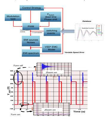
Figure 8. Elaboration of EMI noise sources. Top: principle – Bottom: illustration in the time domain (ideal voltage -red and reconstituted voltage -blue).
