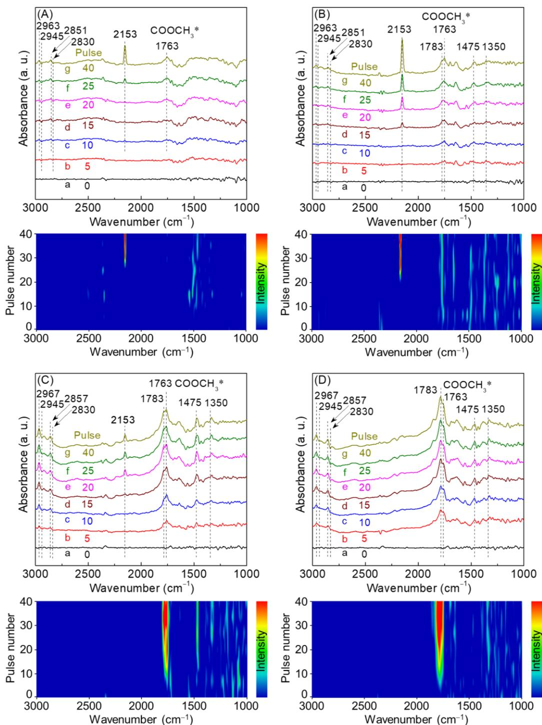
**Fig. 4.** Dynamic changes of DRIFTS spectra on the Pd/NaY catalyst with pre-adsorbed  $\text{CH}_3\text{ONO}$  reactant at (A) 30, (B) 50, (C) 70 and (D) 90 °C as a function of CO pulses: (a) 0, (b) 5, (c) 10, (d) 15, (e) 20, (f) 25 and (g) 40. The sample was pre-treated in  $\text{N}_2$  at 200 °C, cooled down to 30 °C, and exposed to the gas mixture of
