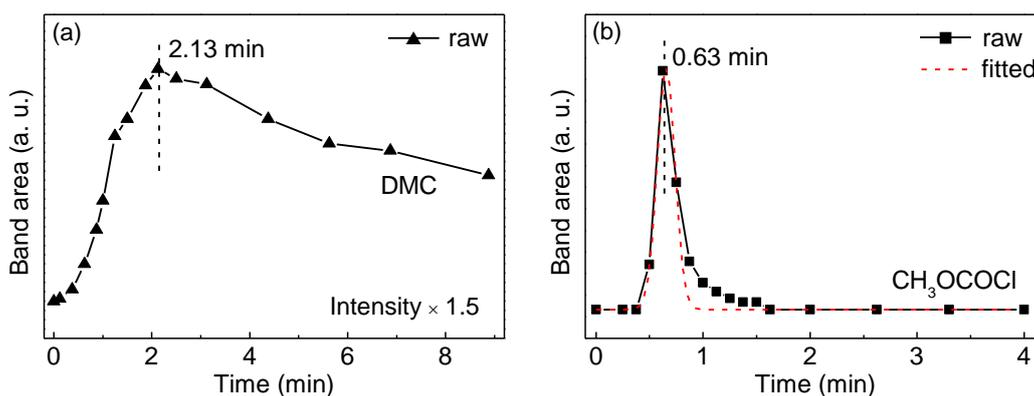
**Fig. 8.** (a) The area of the band at 1780 cm<sup>-1</sup> corresponding to DMC from the DRIFTS spectra presented in Fig. S9A. 3 μL CH<sub>3</sub>OCOCl liquid was injected into the feed gas line and then introduced into the DRIFTS reaction cell with the Pd/NaY
