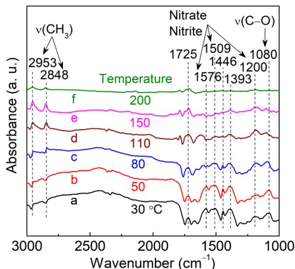
**Fig. 1.** DRIFTS spectra of  $\text{CH}_3\text{ONO}$  adsorbed on the Pd/NaY catalyst at different temperatures: (a) 30, (b) 50, (c) 80, (d) 110, (e) 150 and (f) 200 °C. The Pd/NaY catalyst was pre-treated in  $\text{N}_2$  at 200 °C, cooled down to 30 °C, and exposed to excess of gas mixture of  $\text{CH}_3\text{ONO}:\text{N}_2$  (1: 4; mole) and purged by  $\text{N}_2$ .
