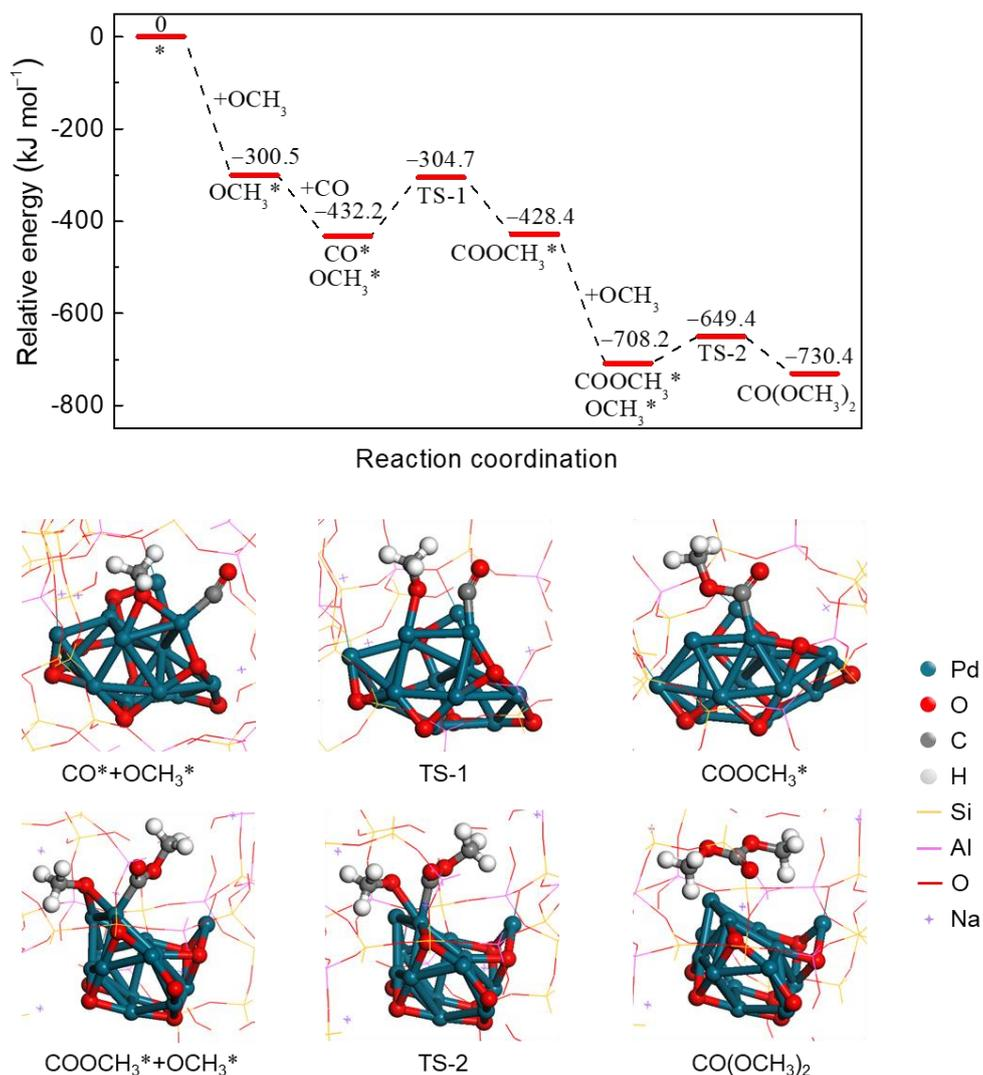
**Fig. 10.** Potential energy diagram for the DMC synthesis from CO and CH<sub>3</sub>ONO together with the related reactant, transition state (TS) and product on the Pd<sub>13</sub>O<sub>8</sub>@NaY model. Blue, red, grey and white spheres represent Pd, O, C and H atoms, respectively. Yellow, pink and red sticks represent Si, Al and O atoms, and purple cross (⊕) represent Na atoms.
