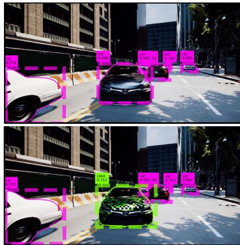
Figure 1: The camouflage fools the Mask R-CNN object detector (on the bottom), whereas plain colors (on top) is being correctly detected (Zhang et al. 2019b).
