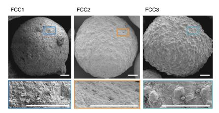
Fig. 1 Electron micrographs of FCC catalysts. Shown are scanning electron micrographs of an FCC1, FCC2, and FCC3 particle. Highlighted is the morphological transition with catalytic deactivation. *Scale bars* are 10 µm
